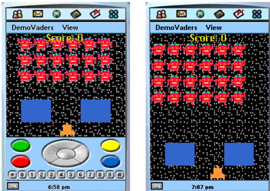
Figure 3 – The UIQ device with the virtual keypad active and virtual keypad hidden.
